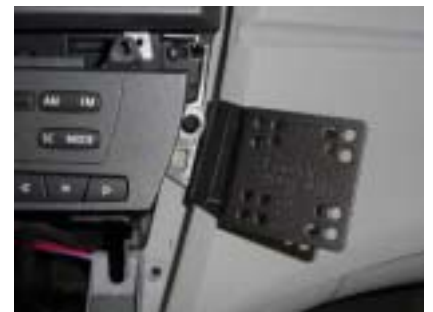
Prototype InDash installed showing screw placement
